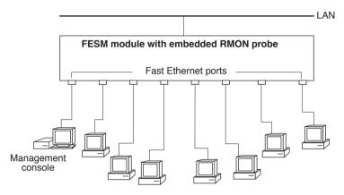
Figure B-2 Embedded RMON Implemented on the CoreBuilder System
